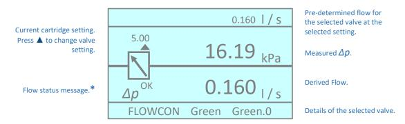
\*If the measured  $\Delta p$  exceeds the minimum required for the selected valve (at the selected setting) to deliver the pre-determined flow, the flow status message will be  $\Delta p$  OK. However, if the required  $\Delta p$  is not present the flow status message will be  $\Delta p$ . In the unlikely event that the measured  $\Delta p$  exceeds the recommended maximum for the valve, the flow status message will be  $\Delta p$ .
