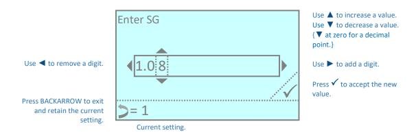
Note: while SG is set to a value other than 1.0, "SG" will show at the top of the chosen display screen as a reminder to the user that readings are being subjected to a correction. It is strongly recommended that users regularly check that the set value for SG is appropriate for the system being commissioned.
