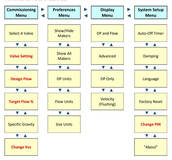
Note: menu options shown in **red** may or may not appear in the menu lists, depending on the selected valve and the precise setup of the handset being used, as follows:
