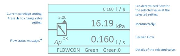
\*If the measured  $\Delta p$  exceeds the minimum required for the selected valve (at the selected setting) to deliver the pre-determined flow, the flow status message will be  $\Delta p$  OK. However, if the required  $\Delta p$  is not present the flow status message will be  $\Delta p$ . In the unlikely event that the measured  $\Delta p$  exceeds the recommended maximum for the valve, the flow status message will be  $\Delta p$ .
