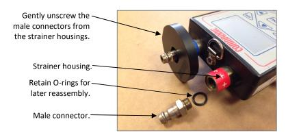
IMPORTANT - Take care not to disturb (i.e. move) the strainer housings. If a male connector doesn't readily unscrew, use a 14mm wrench to hold the strainer housing in place before any additional force is applied.
