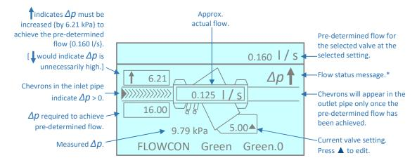
\*If the measured  $\Delta p$  exceeds the minimum required for the selected valve (at the selected setting) to deliver the pre-determined flow, the flow status message will be  $\Delta p$  OK. However, if the required  $\Delta p$  is not present the flow status message will be  $\Delta p$ . In the unlikely event that the measured  $\Delta p$  exceeds the recommended maximum for the valve, the flow status message will be  $\Delta p$ .
