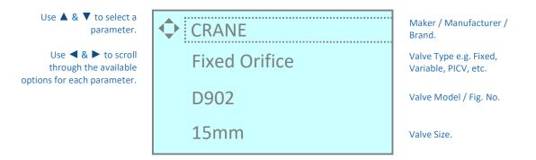
Make selections for <u>all four</u> parameters (i.e. *Maker, Type, Model* & *Size*) before pressing the ✓ button to accept them. Or, press the button to exit and <u>retain the previous selection</u>.
